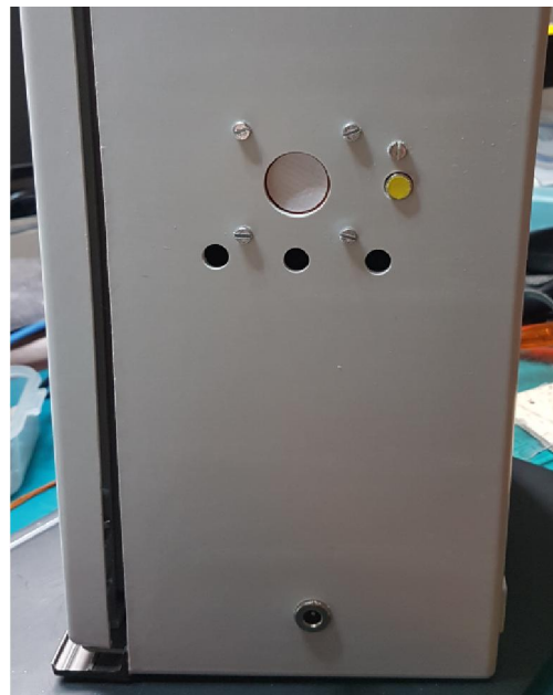
Fig. 7: PM sensor exhaust holes and the installed NO 2 and humidity/temperature sensor, at the bottom the 12V power supply connection
