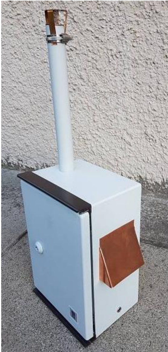
Fig. 5: One prototype of the SMbox measurement unit, on the side wall the copper roof is visible covering the NO 2 and temperature/humidity sensor as well as the OPC sensor exhaust
