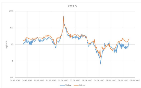
Fig. 16: Un-compensated PM2.5 results of the measurement unit, compared to the reference instrument (28.12. - 06.01.)
