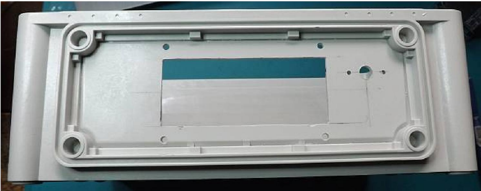
Fig. 12a: Cutouts and holes for the LCD display and the temperature & humidity sensor
