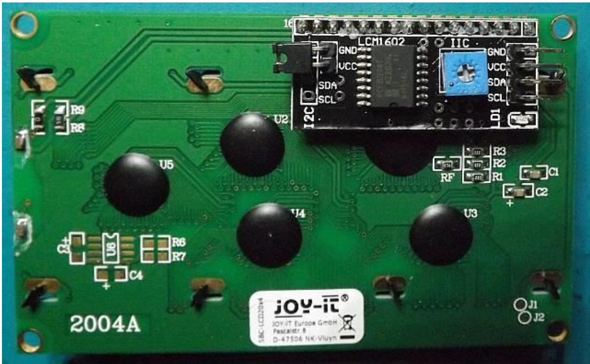
Fig. 6: The backside of the LCD display, it carries a parallel to I2C bus converter piggy-back module
