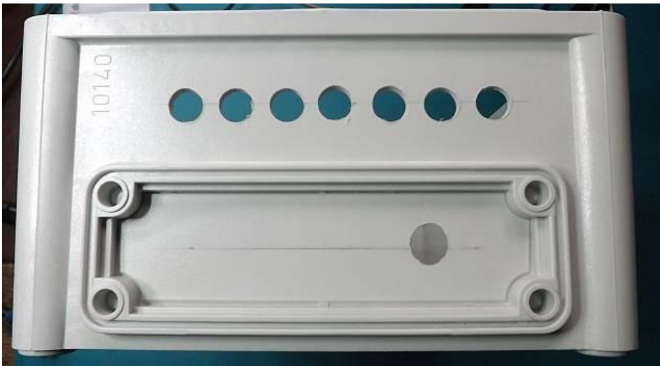
Fig. 12c: Drill holes for the Alphasense OPC air outlet and the external power jack
