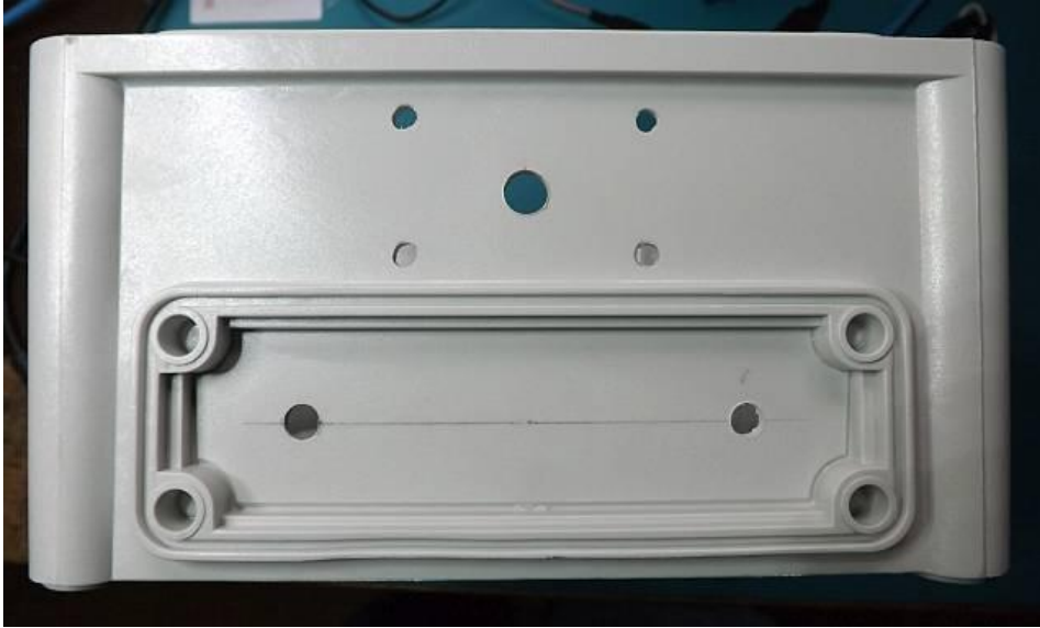
Fig. 12b: Drill holes for the Alphasense OPC, the power and the GPS switch
