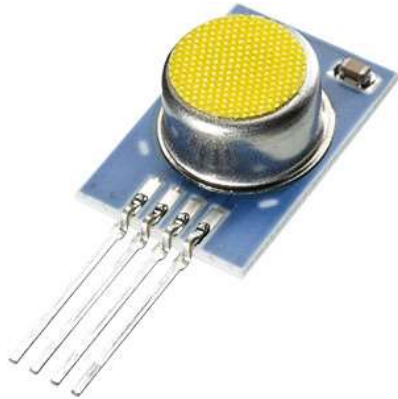
Figure 8: The outdoor capable temperature/humidity sensor HYT221 covered with a protective membrane against wet water and dust
