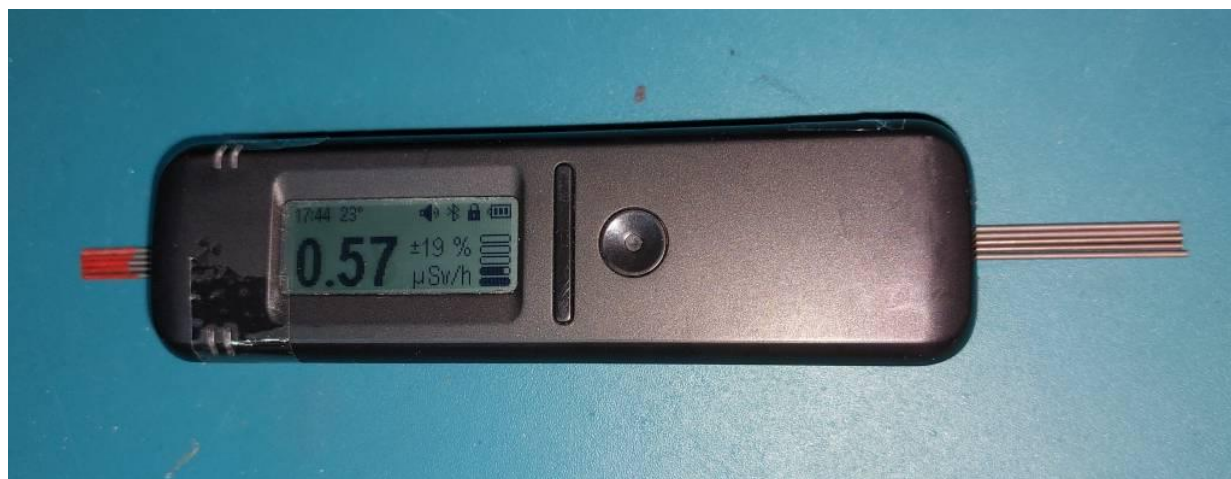
Fig. 11: Thoriated tungsten welding needles measured with the Radiacode RC-101 to obtain a more complex spectrum from Th232 and its daughter products
