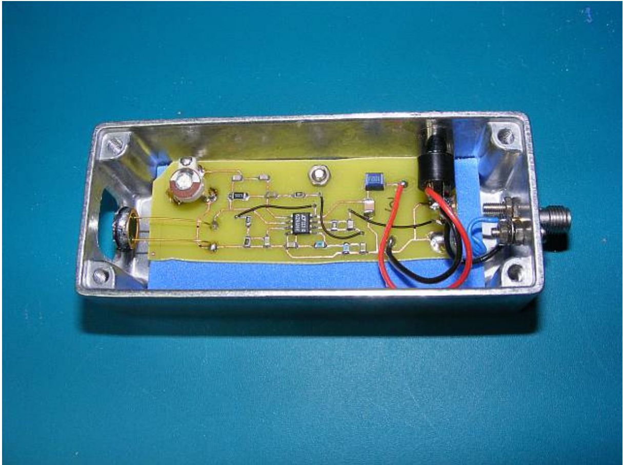
Fig. 2: The interior of the „Mini-Geigerle“ using the S1223 alpha sensitive detector (see separate article)
