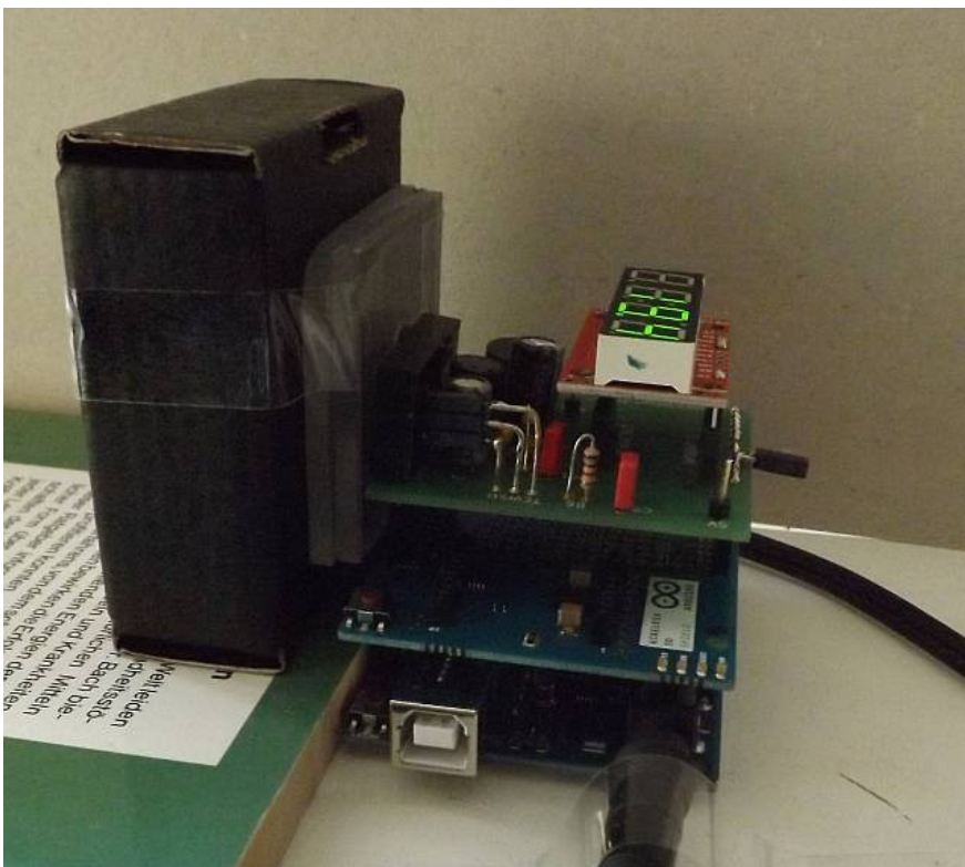
Fig. 7a, b: Measurement with the Tino instrument and recording of the data to a SD-card (located on the middle PCB behind the instrument)
