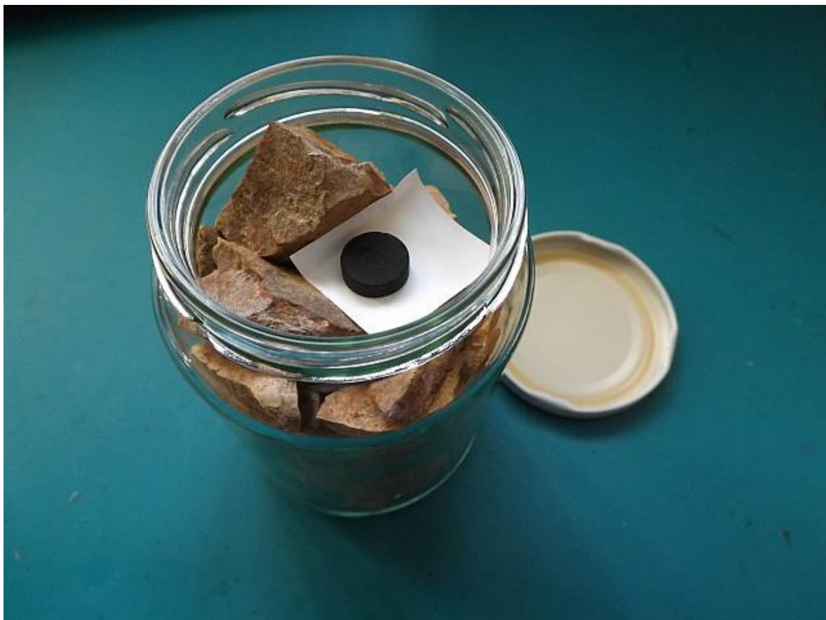
Fig. 1: Jam jar with a porphyry stone sample and an activated charcoal tablet
