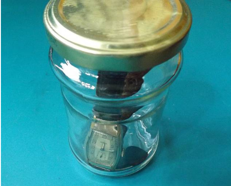
Fig. 10: Wrist watch with radium pointers and an activated charcoal tablet in a jam jar
