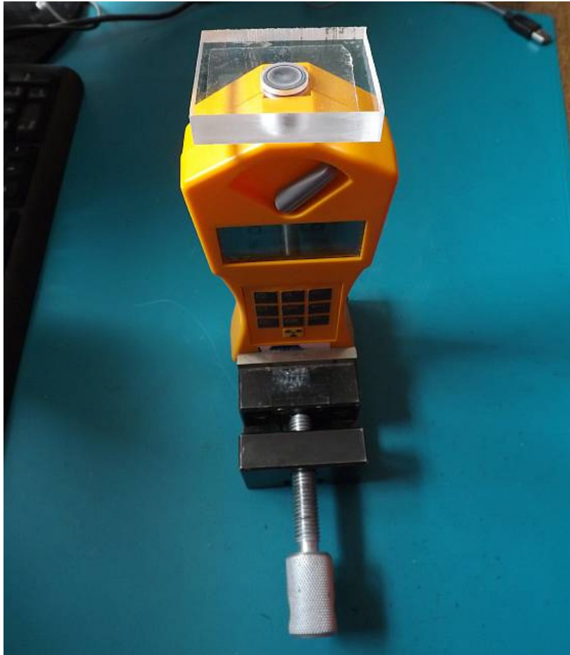
Fig. 4: Through-the-foil measurement using the fixture and a Gammascout
